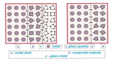
Figure 1: Variants of the structural composition of the metal-quartzcomposite material
